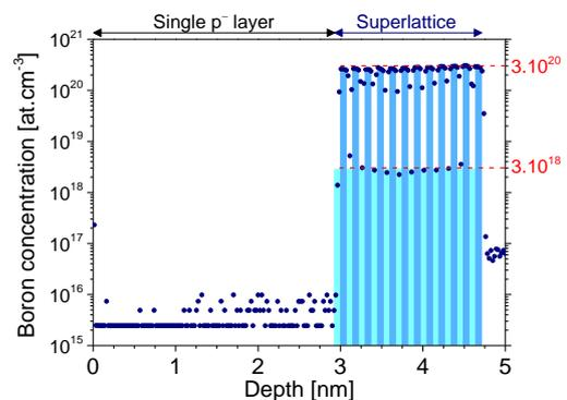
Fig. 1 – Boron concentration in a  $p^-$  layer capping a  $p^{++}/p^+$  superlattice composed of 12 alternate layers measured by SIMS. Blue boxes are visual guides to discriminate  $p^{++}$  and  $p^+$  layers.
